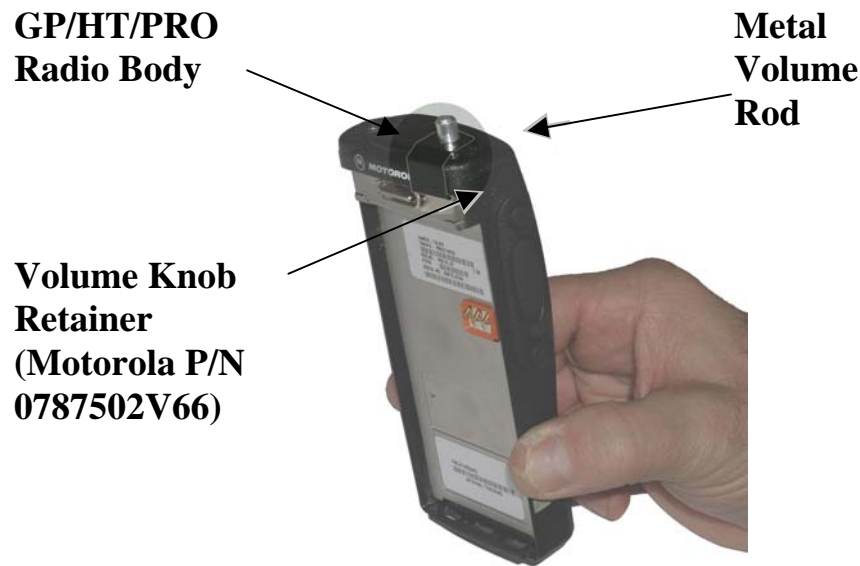
Figure 13-29 Attach Retainer to Radio
